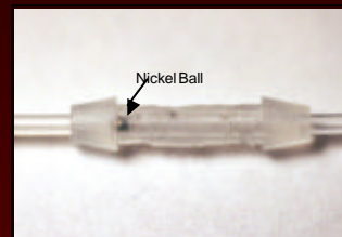
Figure 5. Photographs of micro ball valves before assembling with magnetic actuators. The diameter of the ball is 760 \mu m with 625 \mu m ID x 1190 \mu m OD tubes.
